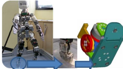
**Figure 2: Robot iCub (IIT) with new variable stiffness: ankle**
