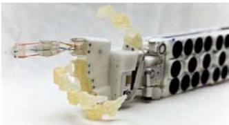
**Figure 2: New hand-arm design with VIA actuators**
