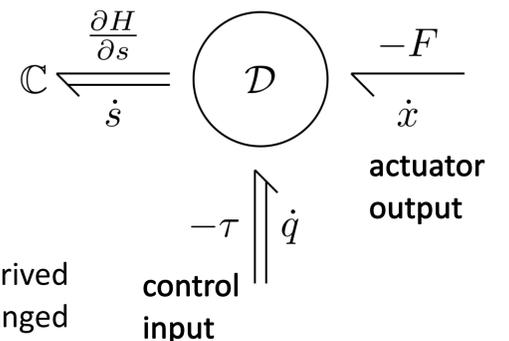
Using this model, design guidelines are derived such that the output stiffness can be changed without supplying energy via the control port.
